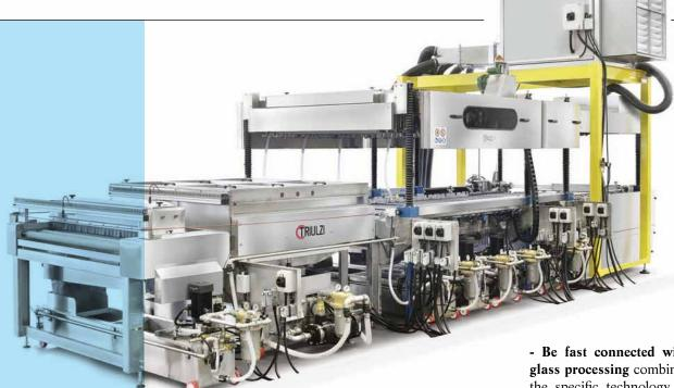
relationship on the specific needs of actual glass producers and the ability to anticipate these needs. Triulzi Cesare Special Equipments Srl produces vertical and horizontal washing and drying machines for flat and curved glass, windshield powder coating systems, ultrasonic cavitation washing systems, lines for treatment of laminated, insulated, etched, or fire-resistant glass.
